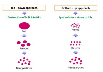
Figure 4. Nanoparticle synthesis methods: top-down and bottom-up approach.
