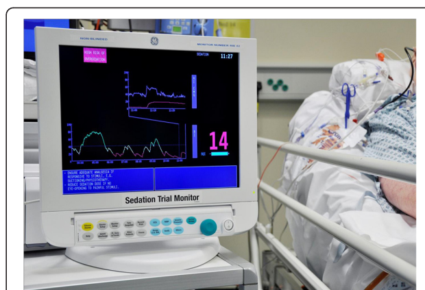
Fig. 1 Responsiveness Index (RI) sedation monitor used in the trial. For intervention patients, the screen presented a running trend over several hours, with the most recent value presented on an arbitrary scale of 0–100, with a colour code of RED ( <20 ), AMBER (20 to 40); and GREEN ( >40 ). In addition to the colour trend, the following prompts were automatically presented according to RI value: RED high risk of over-sedation. Ensure adequate analgesia if responsive to stimuli, e.g., suctioning/physiotherapy. Reduce sedation dose if no eye-opening to physical stimuli. AMBER : moderate risk of over-sedation. Ensure adequate analgesia. Reduce sedation if no eye-opening to physical stimuli. GREEN : low risk of over-sedation. Ensure adequate analgesia. Continue current sedation unless patient agitated
