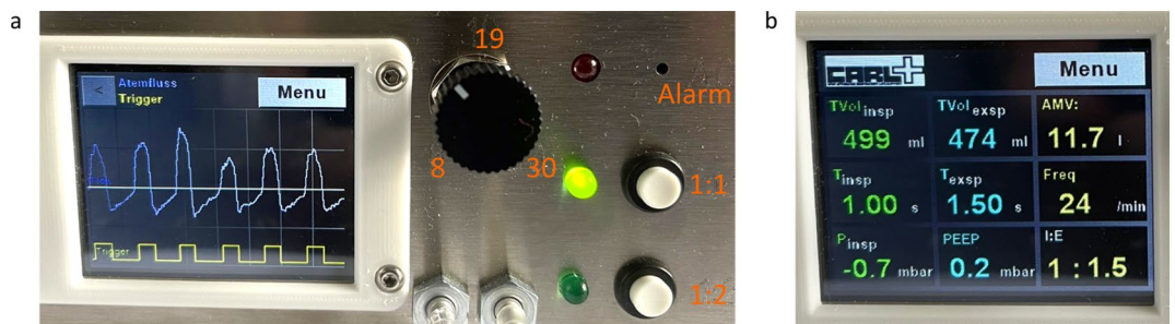
Figure 7. Photo of the user interface of CARL. (a) Entire interface with a display of a flow curve. Ventilation parameters are highlighted in orange. (b) Display of the current ventilation parameters and ventilation quantities.
