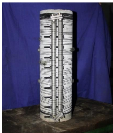
Figure 3. A SMA reinforced concrete cylinder with a wire tensioning and anchoring device.
