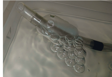
FIGURE 1: Ruptured cuff of the used ETT. When the air was inflated, air bubbles were leaking from the single, ruptured pinhole of the cuff.
