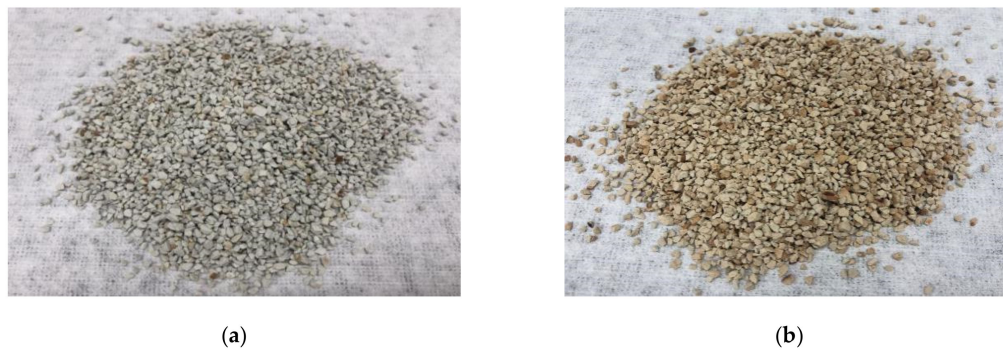
Figure 1. Zeolite sands used to replace standard sand: (a) natural zeolite sand; (b) calcined zeolite sand.
