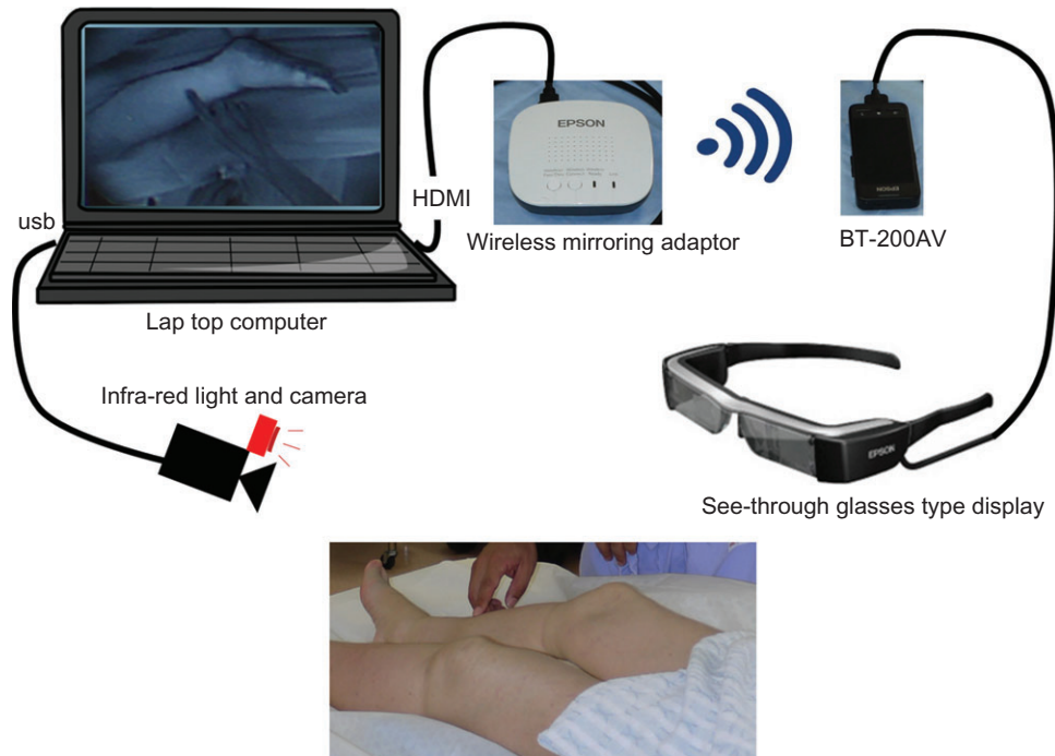
Figure 1: Schematic drawing of the AR system. An infrared light and camera were placed upside down, on the other side of the patient from the operator. A laptop computer was to record and display. Though a mirroring adaptor, the image was wirelessly transmitted and displayed on a see-through glass type display. The operator saw the infrared image overlaid on the real scene.
