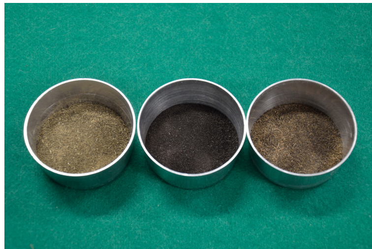
Fig 2. Appearance of raw dairy manure (left), manure treated under air at 90 °C (center), and manure treated under N 2 at 90 °C (right). All samples were dried before being photographed to eliminate the effect of water on the color.
