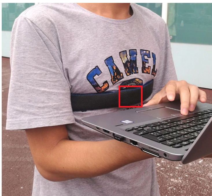
Figure 1. A prototype system of the chest-mounted inertial measurement unit (IMU)-based pedestrian dead reckoning (PDR).
