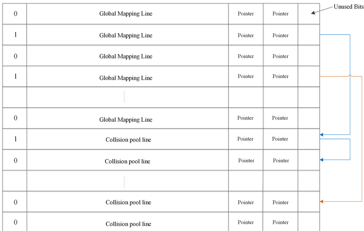
Fig 4. The structure of global ECPs buffer. When valid bit displayed '1', it means these six G entries have already been occupied. we must use the address in pointer area to map to a collision pool line.
