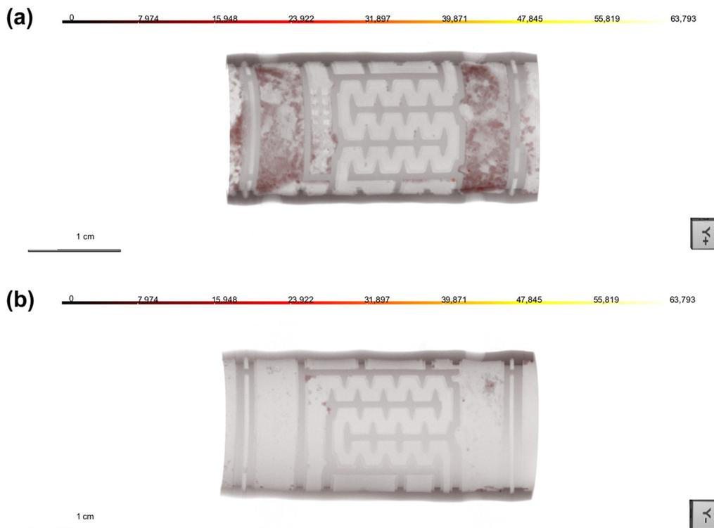
Figure 7. Surface geometry and clogging pattern of sample emitter 4, (a) side 1 and (b) side 2.
