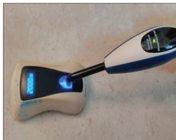
Figure 3: Radiointensity meter from Ivoclar Vivadent – to measure intensity or irradiance of light in mW/cm 2
