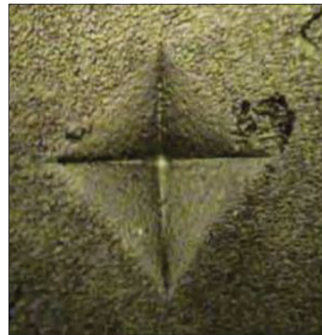
Figure 6: Microscopic image seen at \times 40 magnification of square-based pyramid-shaped indentation formed on resin sample by Vickers hardness indenter
