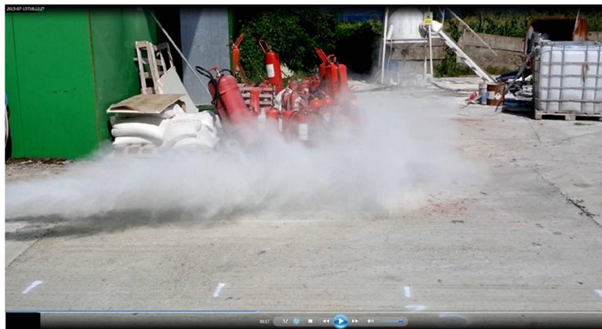
**Figure 21.** Extinguishing jet performance. The fire was maintained by a pile of cotton cloths soaked in liquid fuel or diesel. When the smoke became sufficient and the wind direction changed toward the robot, the smoke sensors triggered the fire extinguishing system. The system was constructed with the help of two inert gas fire extinguishers.
