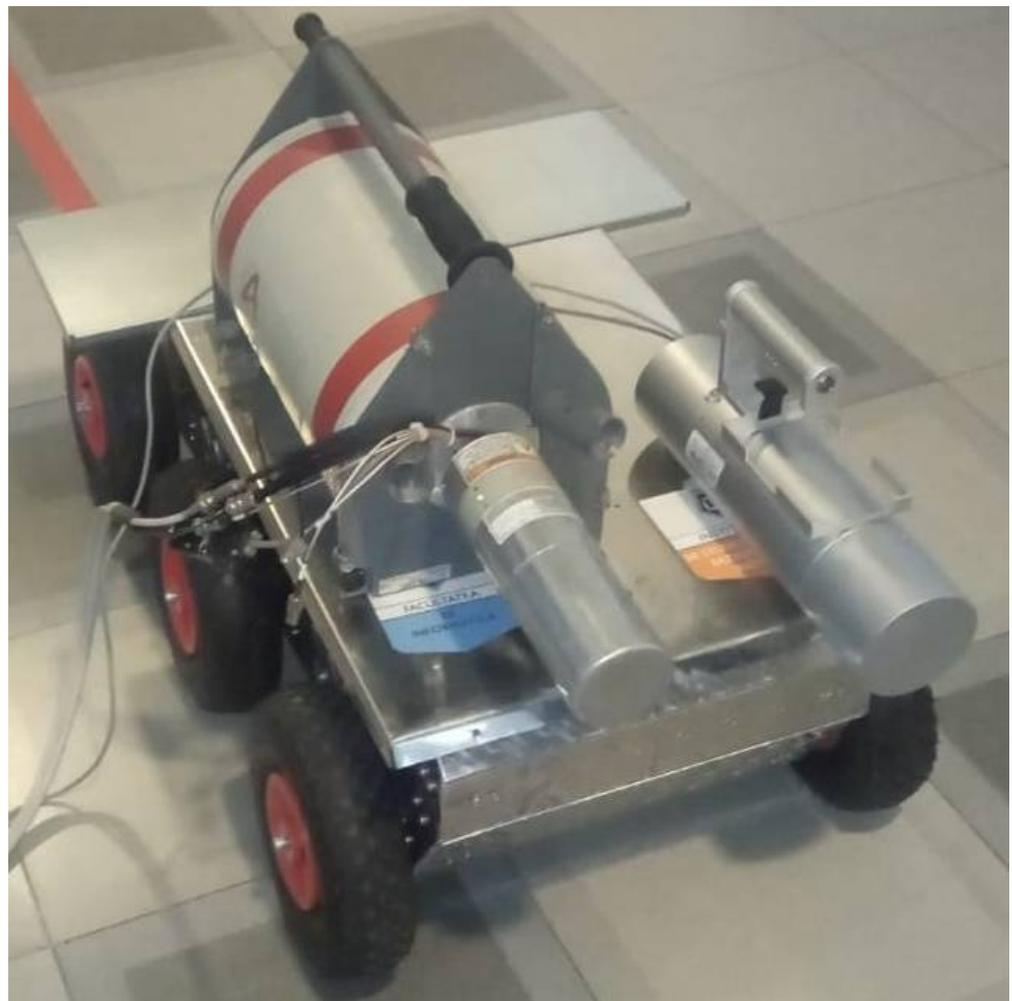
**Figure 25.** Robotic system with an operational vector used to determine gamma radiation. The experiments were recorded at Titu Maiorescu University in Bucharest.
