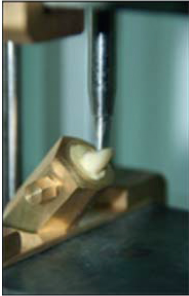
FIGURE 13: Loading stylus applying load onto the palatal surface of the crown 135° to the long axis of the tooth during the fracture resistance test.
