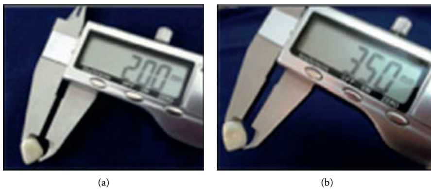
FIGURE 4: Checking thickness of the finished CAD/CAM zirconia all-ceramic crown: (a) all-ceramic crown of 2 mm incisal thickness; (b) all-ceramic crown of 3.5 mm incisal thickness.
