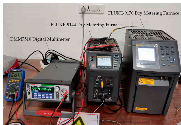
Figure 10. A thin film thermocouple temperature sensor static calibration system.
