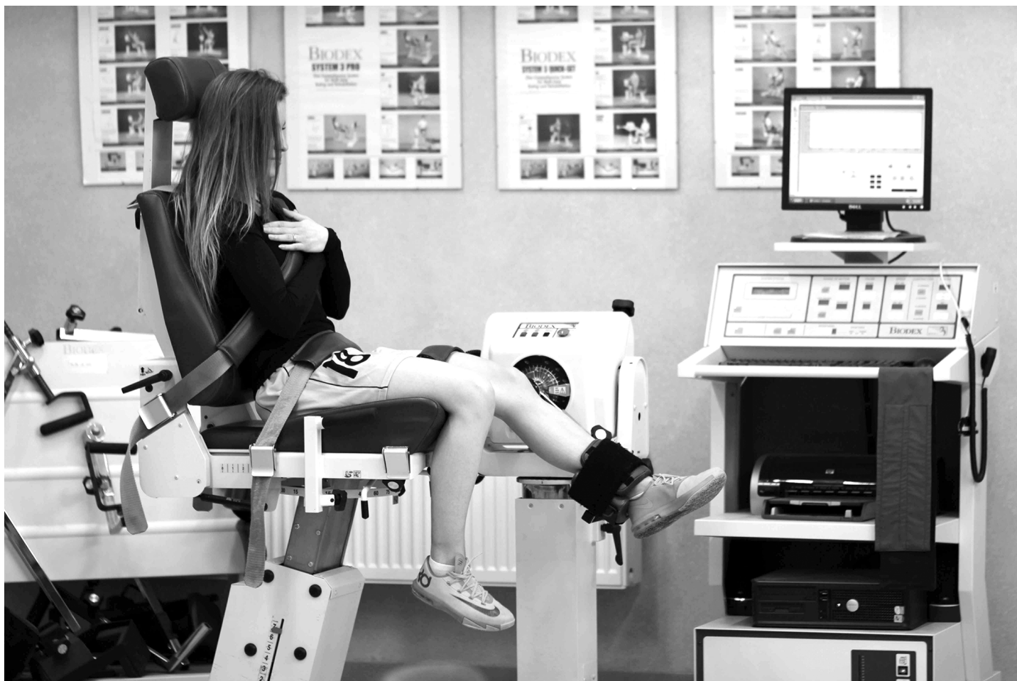
Fig 1. Test of the concentric isokinetic quadriceps and hamstrings torque on the Biodes 3 System.
