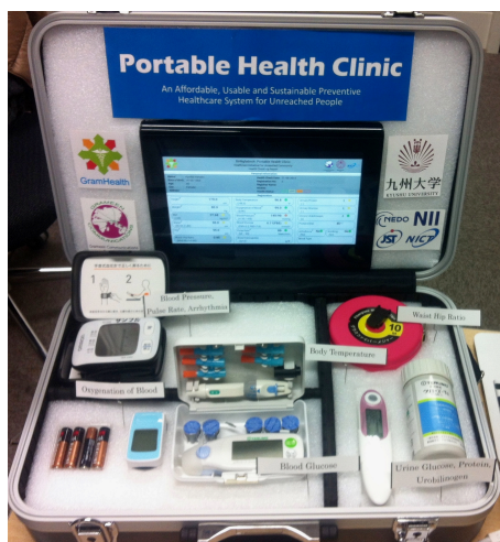
Figure 1. Sensors inside the Portable Health Clinic Box.
