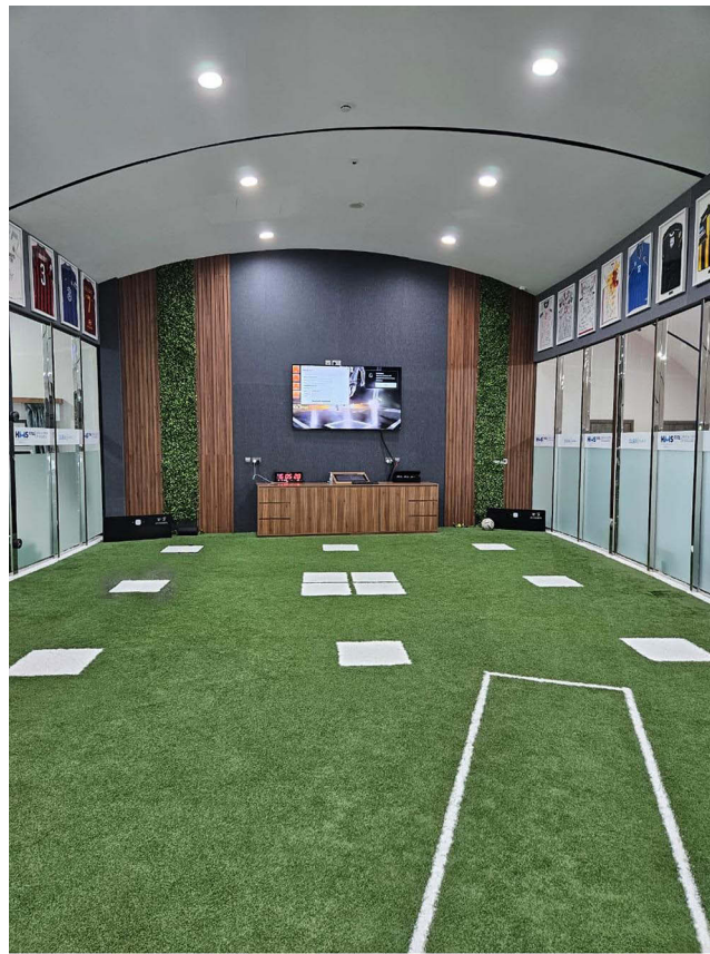
Figure 1 Speedcourt System consisting of a platform (5.0 × 5.0 m) with 12 contact sensor plates positioned in symmetrical order.
