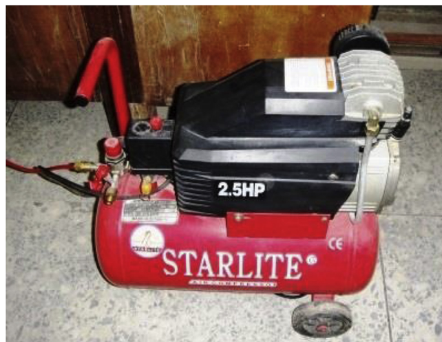
Figure 10. Air compressor pump.
