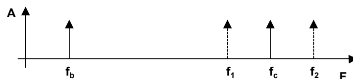
Figure 7. Spectrum of the sum of two sinusoidal functions having frequencies f_1 and f_2 and the resulting carrier and beat frequencies f_c and f_b , respectively.
