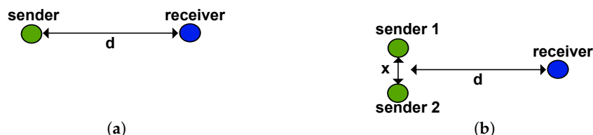
Figure 20. Schematics of the experimental setups for (a) single wake-up and (b) concurrent wake-up.
