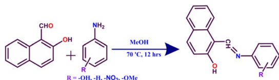
Scheme 1 Synthetic pathway of 2-hydroxy naphthaldehyde derivatives (N1, N2, N3, N4, and N5).
