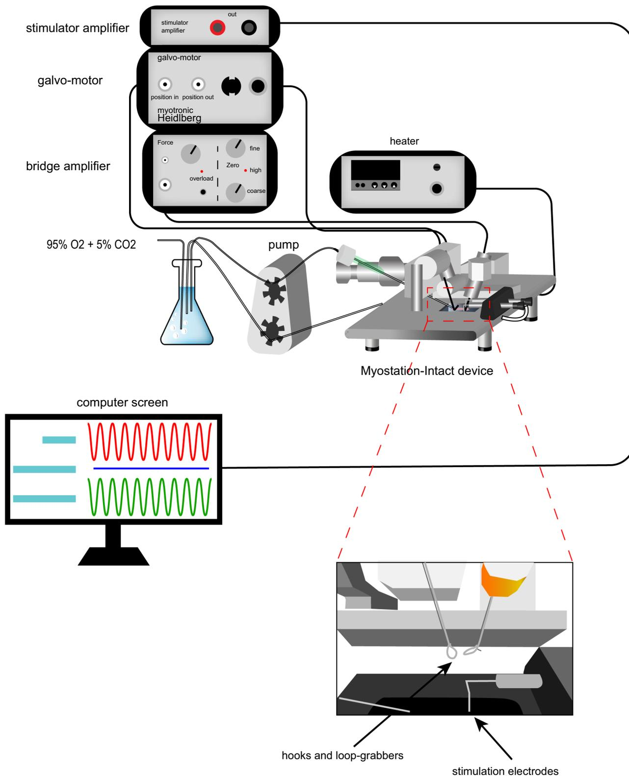
FIGURE 1 Schematic graph of Myostation-Intact system
