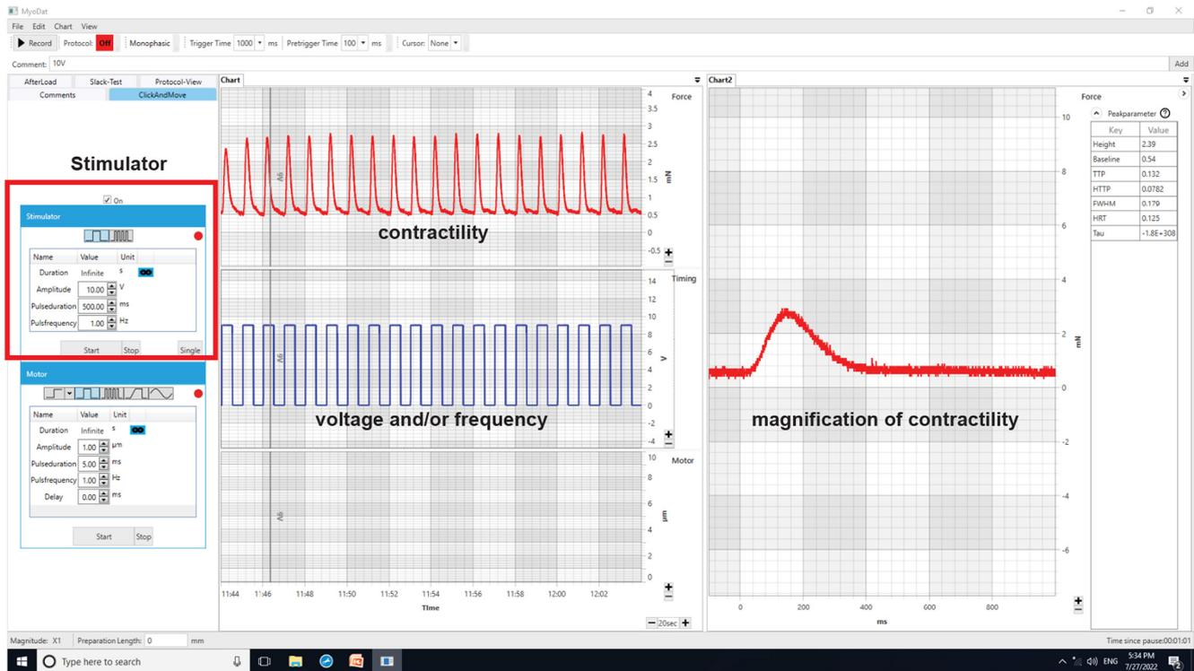
**FIGURE 3** Interface of MyoDat recording software on computer screen. The red rectangle box in the left panel includes the stimulation parameters: voltage, duration, and frequency. The middle upper panel shows the contractility, and the lower panel shows the stimulation of voltage and frequency. The right panel shows the magnification of the contraction force
