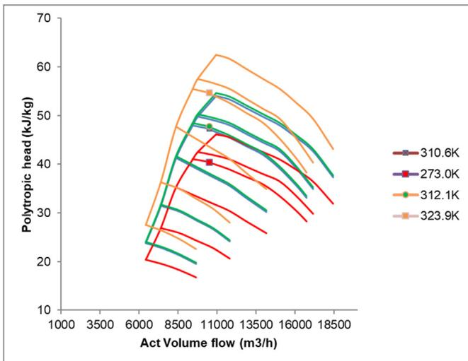
Figure 7. Polytropic head reference point changes in Centrifugal Compressor map due to Ambient temperature.
