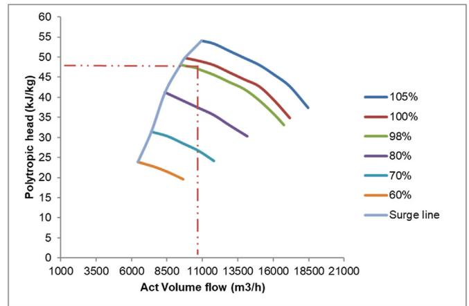
**Figure 1.** Centrifugal compressor characteristics showing the polytropic head against the actual volumetric flow.
