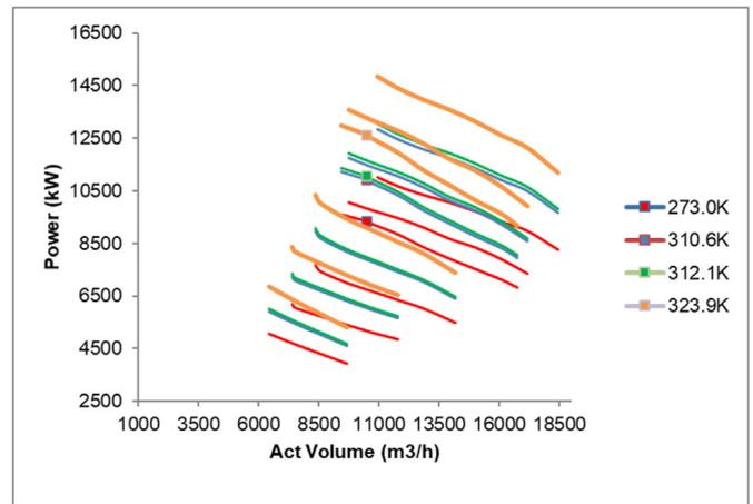
Figure 8. Power demand reference point changes in Centrifugal Compressor map due to Ambient temperature.
