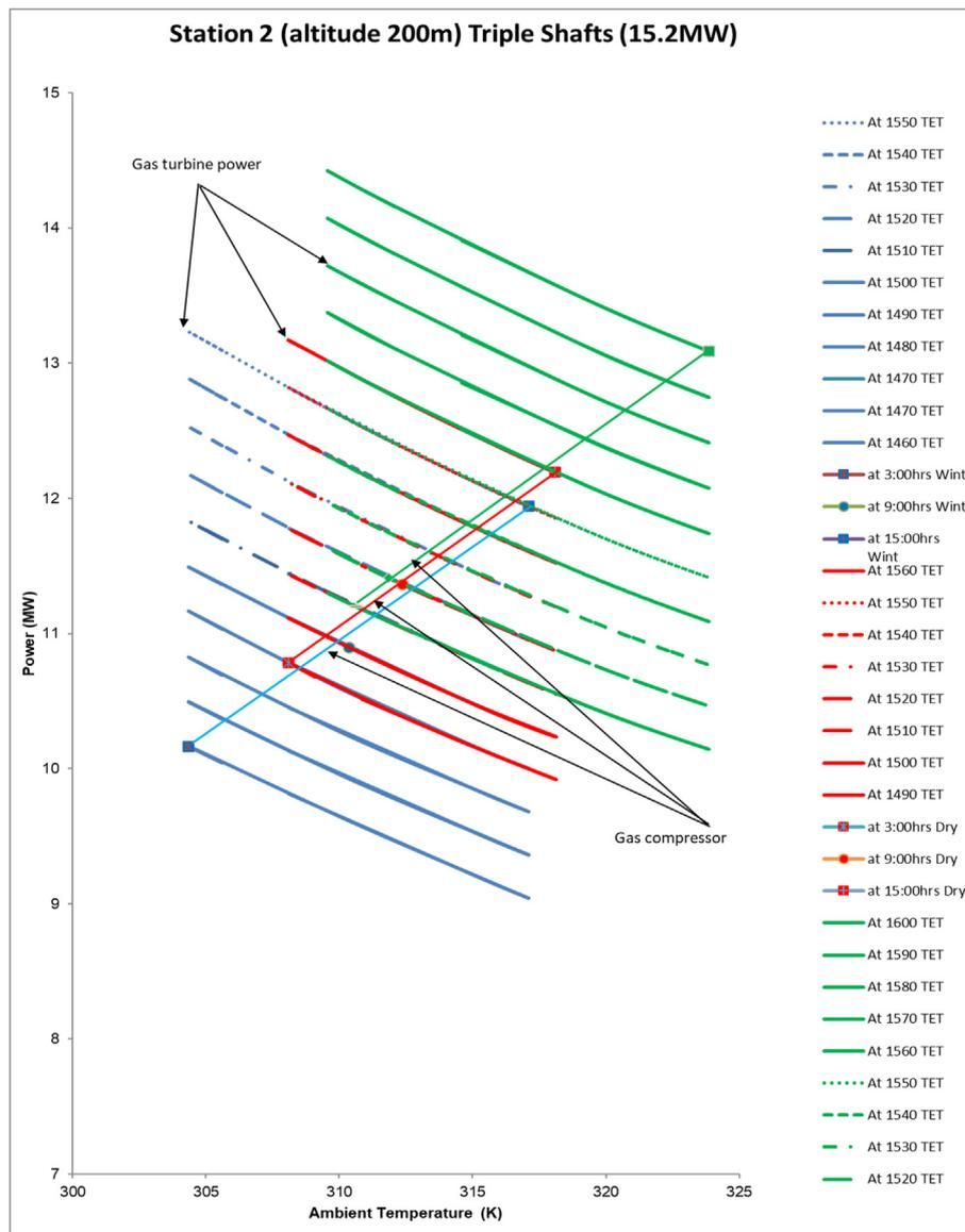
Figure 11. Gas compressor & Gas turbine power matching.
