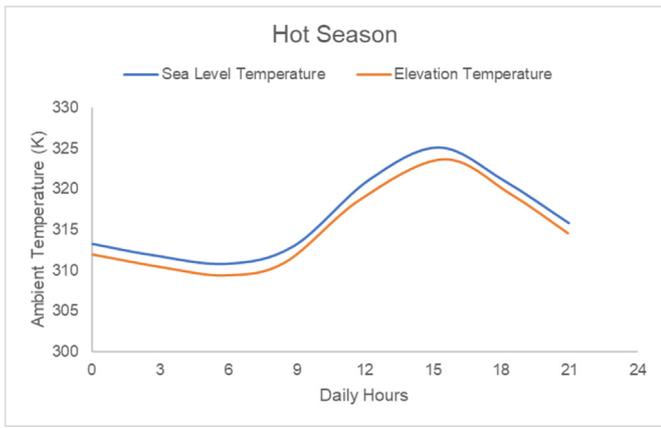
Figure 5. Ambient temperature curve at compressor station 2 during the hot season.
