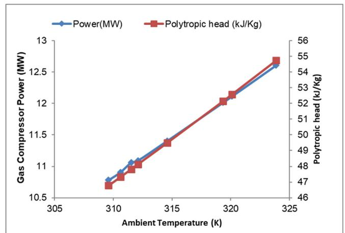
Figure 9. Effect of Ambient temperature on compressor performance.
