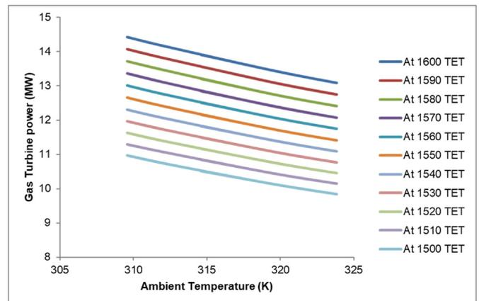
Figure 10. Effect of ambient temperature on gas turbine power.
