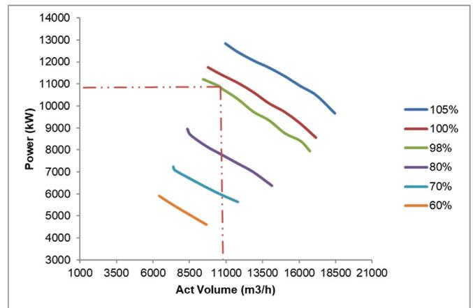
**Figure 2.** Centrifugal compressor characteristics showing the power demand against the actual volumetric flow.
