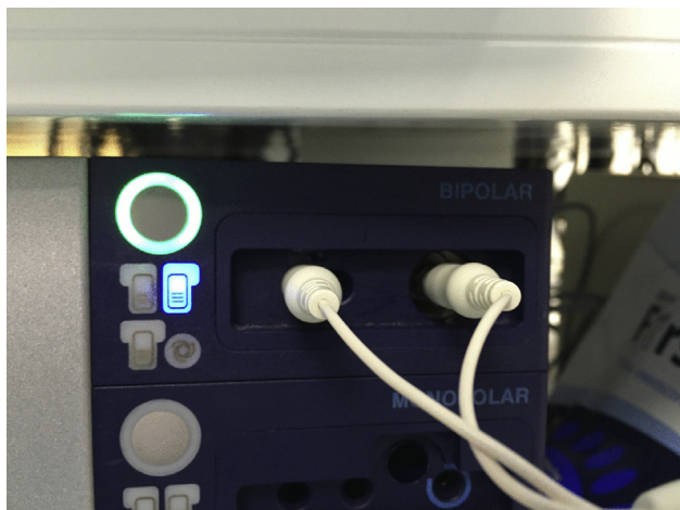
Figure 4. Proper installation of bipolar system: cord from bipolar device placed into uppermost bipolar portion of electrocautery system.
