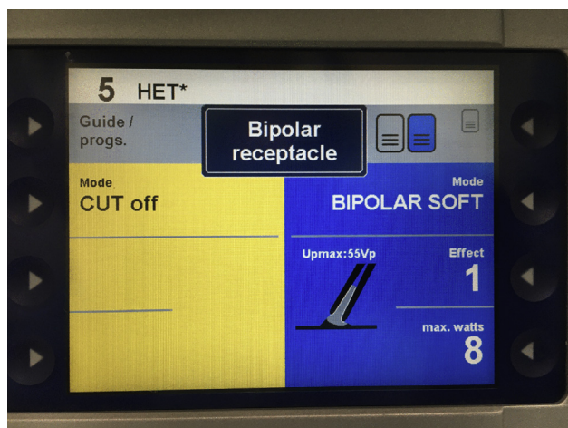
Figure 5. Electrocautery setting for bipolar system. Visible monitor reveals bipolar setting of electrocautery system at effect 1, 8 W.
