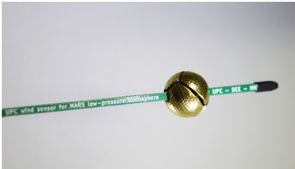
Figure 1. Photograph of the 4-sector spherical sensor (10 mm diameter), before being wrapped and inserted into the regolith simulant.
