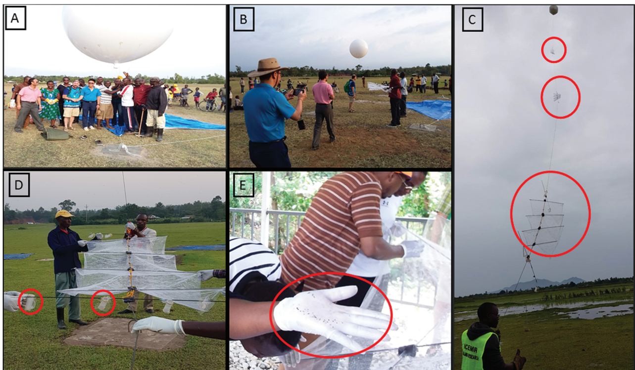
Fig. 2. A) Launching tethered balloon. B) Fixing the sticky panels on the tethered string. C) Tethered balloon with 3 sticky panels at heights 9, 120, and 160 m agl. D) Sticky panel and open ended suspended falcon tubes containing mosquitoes exposed to high-altitude condition. E) Collecting and sorting captured insects.
