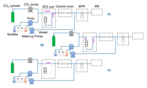
**Figure 2.** Scheme of the supercritical fluid extraction-supercritical fluid chromatography-mass spectrometry (SFE-SFC-MS) system: **(A)** Static extraction mode, **(B)** Dynamic extraction mode, **(C)** Analysis mode. Reprinted with permission from [17].
