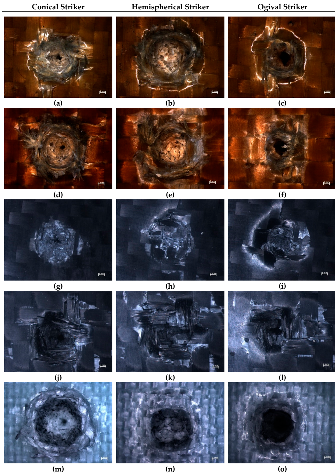
Figure 5. Microscopic images of damage caused by the strikers with various geometry in the epoxy composites with reinforcement made from the following fibers: (a–c) Twaron 2200, (d–f) Kevlar 49, (g–i) Pyrofil TR30 S, (j–l) HR 12K, (m–o) Dyneema SK 60.
