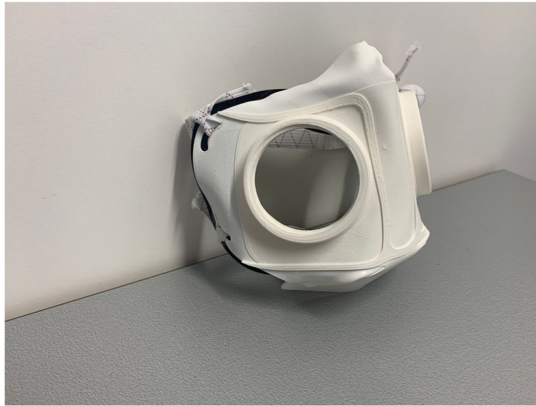
Fig. 5 Side view HSU/BwKWST FM V3. Thermoformed face mask in version three with elastics and TPU sealing lip, black
