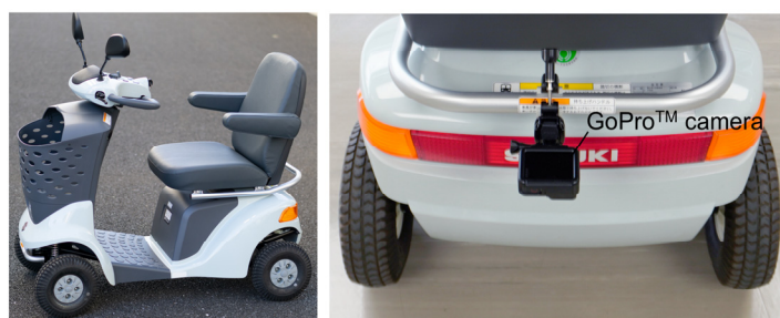
Figure 1. Motorized mobility scooter equipped with a monocular camera.
