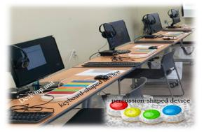
**Figure 2.** Basic settings of devices. Therapeutic musical devices comprise a desk-top unit, monitor, speaker, headphone, and percussion- and keyboard-shaped electrical devices on the desk.
