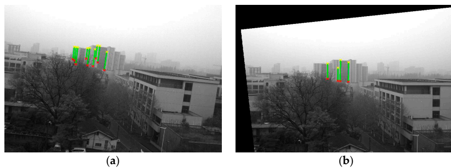
Figure 9. Images with detected plumb lines before and after horizontal correction in System 1. (a) The original image I_3 ; (b) The horizontally corrected image I_{3\_corrected} .
