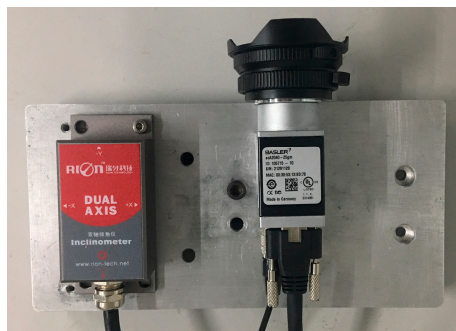
Figure 7. The photoelectric measurement system (System 2) by the Basler acA2040-25gm camera and the SCA126T inclinometer.
