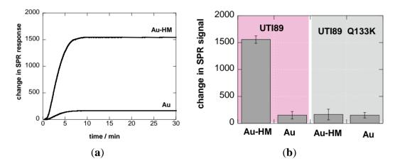
**Figure 2.** (a) SPR sensogram of affinity interaction of *E. coli* UTI ( $10^8$  cfu/mL) with Au and Au-HM interfaces; flow rate = 20 µL/min; (b) bar graph diagrams of the change in SPR signals of Au and Au-HM interfaces upon interaction for 30 min at a flow rate = 20 µL/min with UTI 89 and UTI89 Q133K.
