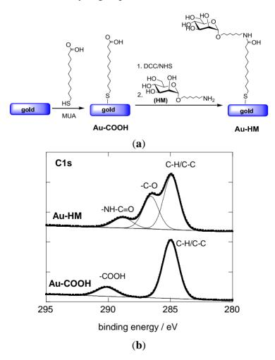
**Figure 1.** (a) Reaction scheme for the formation of aminoheptyl  $\alpha$ -D-mannopyranoside modified SPR interfaces; (b) C1s core level XPS spectra of Au-COOH and Au-HM interfaces.
