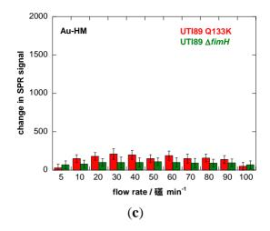
**Figure 3.** Binding affinity of *E. coli* UTI89 ( $10^8$  cfu/mL) to Au and Au-HM as a function of flow rate. (a) Bar graph of change in SPR signal upon addition of *E. coli* UTI ( $10^8$  cfu/mL); (b) SPR sensogram for three different flow rates; (c) binding affinity of *E. coli* UTI89 Q133K ( $10^8$  cfu/mL) and UTI89  $\Delta fimH$  ( $10^8$  cfu/ml) to Au-HM surfaces as a function of flow rate.
