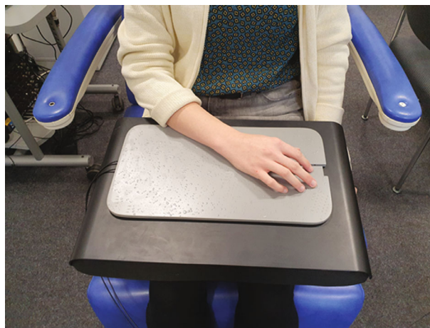
FIGURE 1: Experimental set-up. The participants were comfortably seated in a reclining chair, and the tapping board was placed on the participants' thigh. Tap-onsets were registered by means of a photoelectric barrier mounted on the tapping board (Elekta Neuromag®, Helsinki, Finland).
