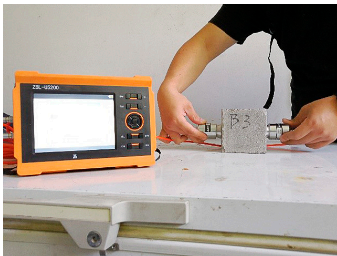
Figure 10. The measurement of ultrasonic pulse velocity of concrete specimen.
