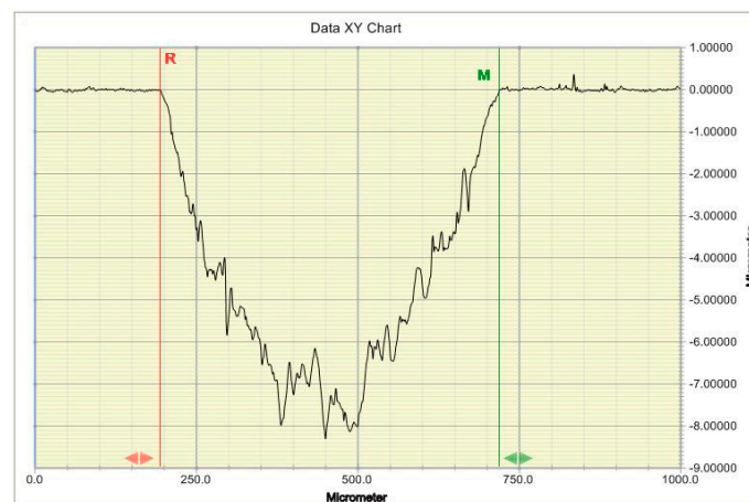
Figure 4. Typical 2D profile of dental material wear mark.
