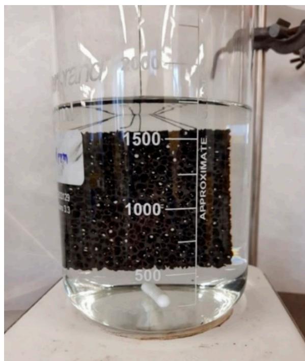
Figure 1. Sorption experiment of the coated ceramic foam filter.
