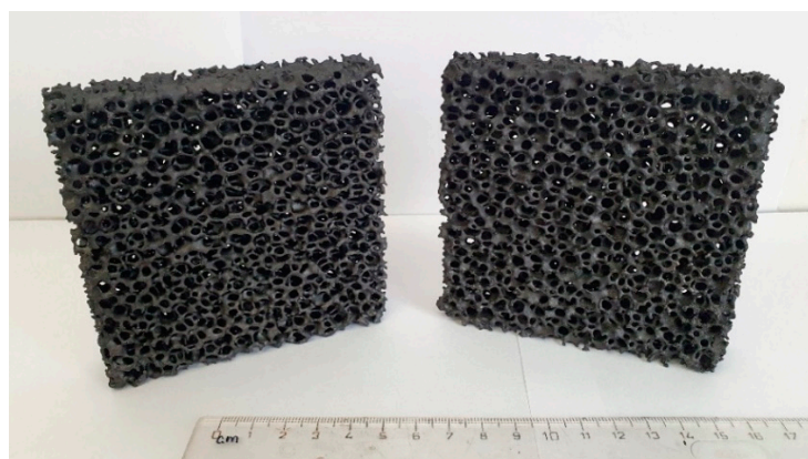
Figure 6. Photography of ceramic foam filters before the dip-coating (left) and after the dip-coating (right).
