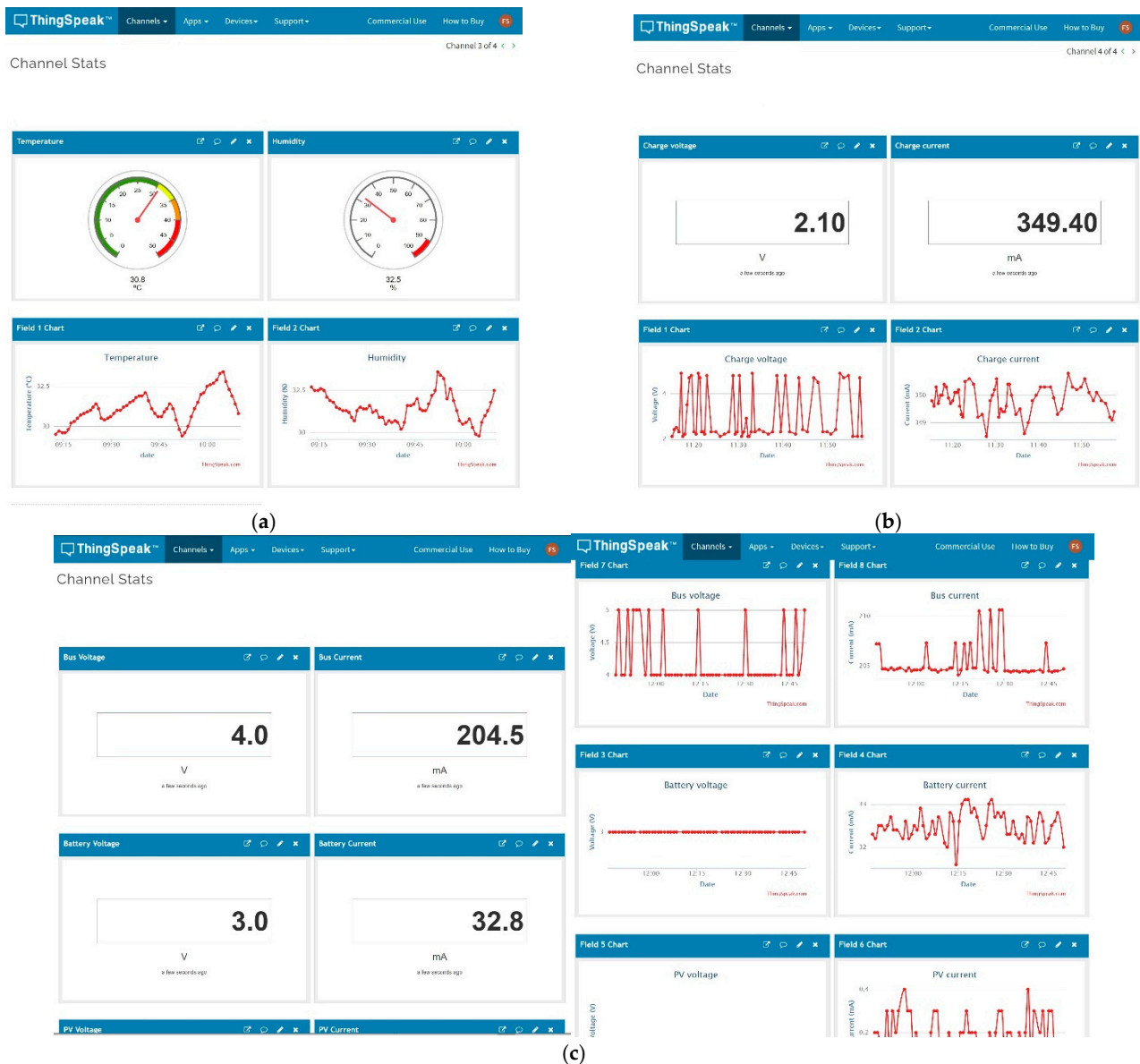
Figure 26. ThingSpeak Integration: (a) temperature and humidity data; (b) battery USB charge; and (c) THMDL battery power supply operation.
