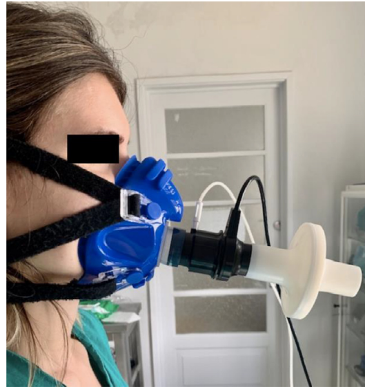
Fig. 1 Filter placed in-line and downstream of the gas analyzer sample.
