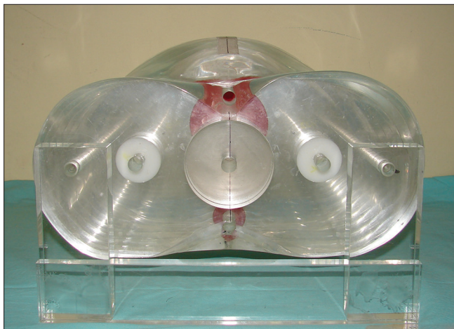
Figure 4: Pelvic phantom transverse view with CC01 ionization chamber slots
