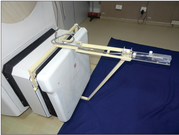
Figure 2: Metallic mount (with ionization chamber in transit position) fixed to electronic portal imaging device of linac
