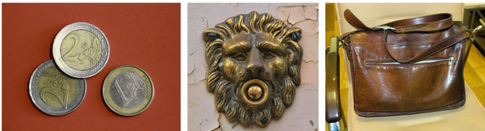
Figure 1. The occurrence of spatially-varying reflection characteristics on a surface can be due to several causes: Many objects are made of different materials, such as the Euro coins in the left image which consist of two parts with different metal alloys. Some surfaces are partly covered with layers of impurities, such as patina (center image). Other materials, like leather (right image), are comparatively sensitive to mechanical influences and can be easily roughened or polished which may locally affect their light reflecting behavior. (All images were taken from pixabay.com.)
