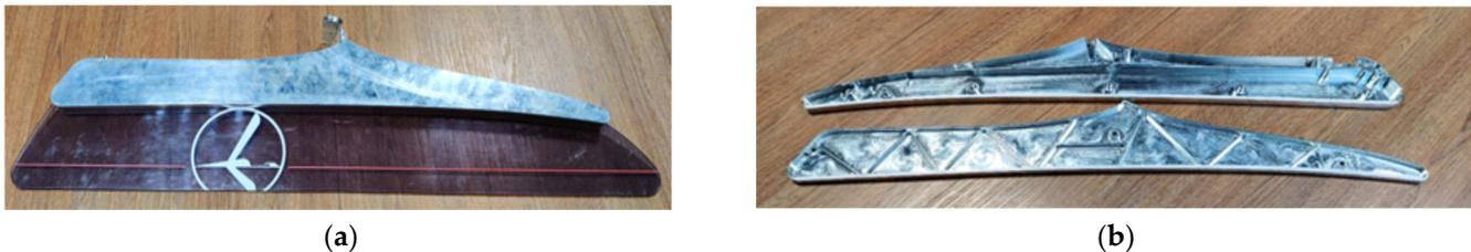
**Figure 4.** Class-divider part: (a) assembled, and (b) inside view of the two halves of the class divider.
