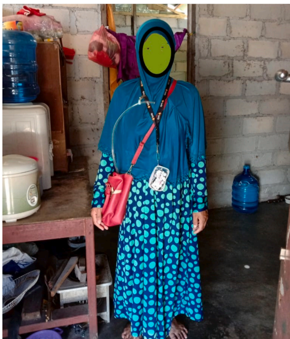
Fig. 2. A respondent carried instruments in a bag, with the inlet tube placed in the breathing zone and exposed to the air.
