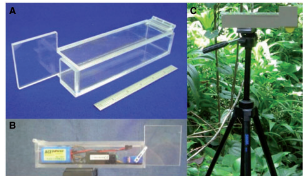
Figure 2. Dewlap display apparatus. (A) Acrylic box within which electrical components were placed. The rule next to the box is 15.25 cm in length. (B) Electrical components inside the acrylic box with a fake dewlap displayed. (C) The apparatus in the field with a fake dewlap displayed.
