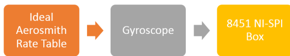
Figure 22. SFNL Test Block Diagram. SPI Box is used to acquire the Gyroscope reading sent from the ASIC through SPI protocol. Rate Table is used to apply angular velocity on the gyroscope.
