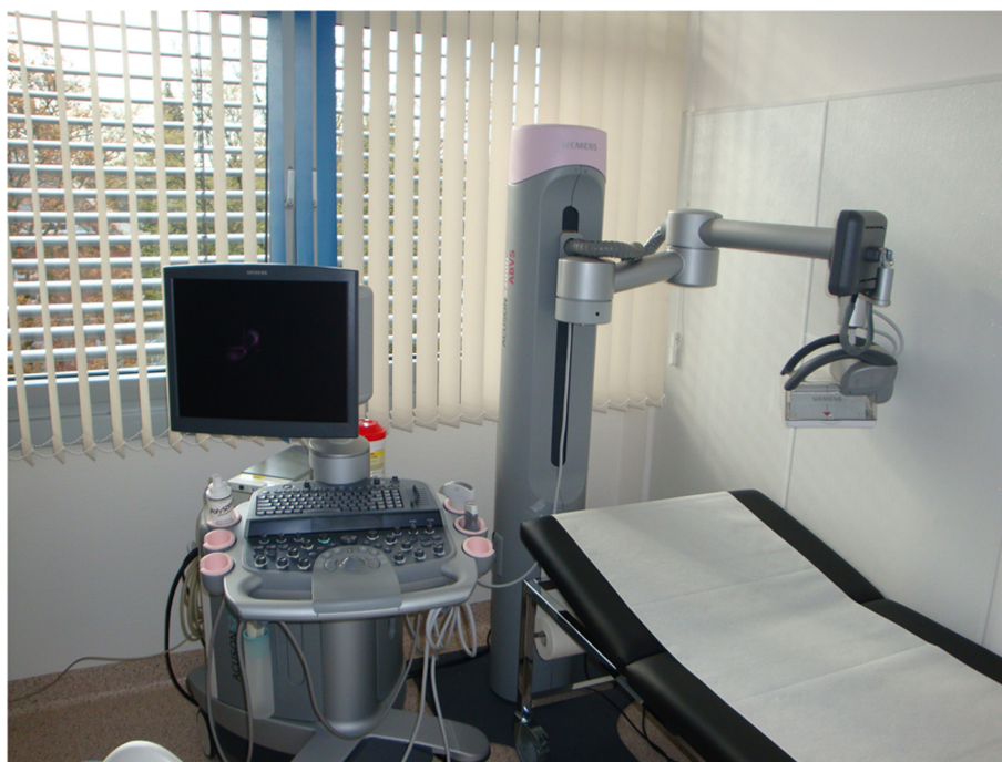
Figure 1 ACUSON S2000 ™ ABVS. On the left-hand side is the ACUSON S2000 ™ ultrasound machine, on the right-hand side is the 14L5BV volume transducer attached to a mechanical arm.
