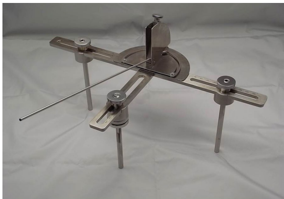
Fig. 1 The HipCOMPASS mechanical intraoperative angle guide device. The device has legs to be placed on the left and right anterior superior iliac spines (ASIS) and on the pubic symphysis. The width to the left and right ASIS and the height to the pubic symphysis are variable, and adjusted to each individual patient. The length of the leg placed on the pubis is also adjustable, allowing for the correction of angle errors caused by soft tissue. The left and right ASIS legs are hollow, and the device is fixed to these ASIS by the insertion of Kirschner wires through them from above. An angle indicator is placed on the device, and the cup is inserted parallel to the direction of the indicator, thereby increasing its accuracy
