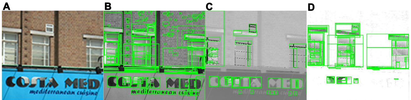
Fig 2. Multi-channel MSER components extraction. (A) Original image [53]. (B) MSER on gray channel. (C) MSER on PII-hue channel. (D) MSER on PII-sat channel.
