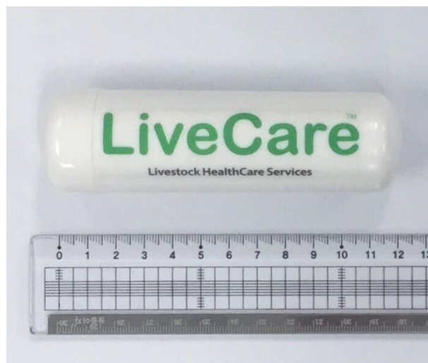
Fig. 1. The Biocapsule including the 3-axis acceleration and temperature sensor.
