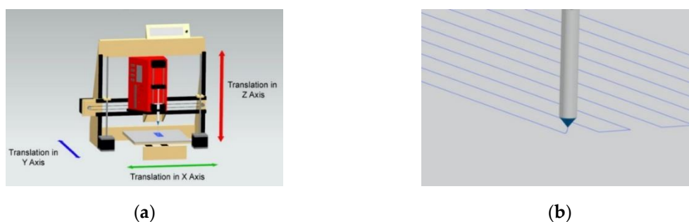
Figure 1. (a) Schematic of a custom modified three-dimensional (3D) printer used to create the NFES apparatus. (b) Representative depiction of precisely written NFES fibers.
